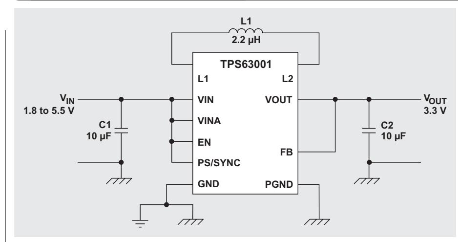
external part count reduces the total solution size to only  $6 \times 6$  mm (see Figure 3).
