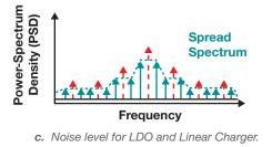
Figure 3: Typical spurious frequencies and noise.
