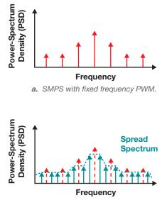
b. SMPS with power-saving PFM or spread spectrum mode.
