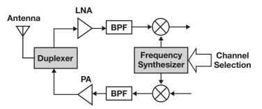
Figure 1: A typical RF tranceiver diagram.
