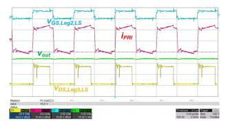
*Figure 5.* Steady-state waveform of a PSFB converter with a center-taped rectifier and active snubbers at a 12-V/3-kW output.
