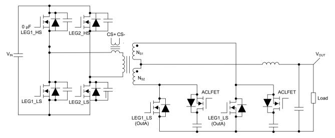
Figure 4. A PSFB converter with active snubbers on a center-taped rectifier.
