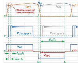
Figure 1. A PSFB power stage with a passive clamp and key waveforms.
