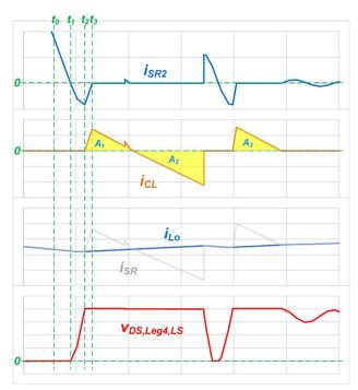
Figure 3. Key waveforms around the active clamp current conduction period.
