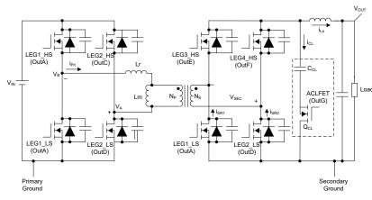
Figure 2. A PSFB power stage with active clamp and key waveforms.
