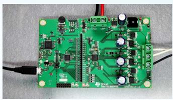
Industry's first automotive BLDC gate driver operating at cold crank voltages as low as 4.4V. This device enables the pump to push fluid in low voltage conditions.
