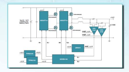
The TIDA-00705 is an ultra-compact (1"x1"x1") high efficiency bi-directional DC-DC power converter capable of delivering 480W for use in Local Energy Storage (LES) and Battery Back-up power applications, specifically designed for server PSUs embedded with battery backup units (BBU).
