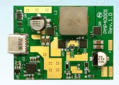
A wide variety of USB Type-C<sup>™</sup> demonstrations are on display, showcasing Tl's versatility and ability to address any application. Multiple automotive USB Type-C<sup>™</sup> designs include key features that any automotive power supply designer would lovehigh efficiency, high switching frequency, low EMI, low Iq, and wide input voltage.
