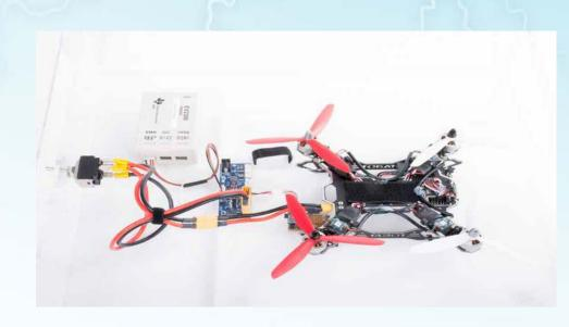
Add flight time and extend battery life to quadcopters and other non-military consumer and industrial drones used to deliver packages, provide surveillance or communicate and assist at long distances. This live demonstration and interactive GUI shows TI technology monitoring the drone's battery in real time - including state of charge, remaining time to empty, and the battery's state of health.
