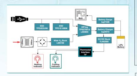
The demo utilizes TI's 24Vac reference designs to provide power and backup functionality to a WiFi-enabled smart thermostat, which can be controlled with a phone. Two lights representing a heater/furnace and cooler/compressor are displayed. When the thermostat's desired temperature is adjusted, the demo will light up the appropriate light to indicate cooling or heating.
