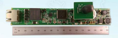
In the era of IoT, Texas Instruments has developed PMP20537, a IEEE802.3bt compliant Power over Ethernet Powered Device (PoE PD) system solution for smart lighting and IoT applications such as energy management, reactive room illumination, wayfinding, and alert/alarm systems.
