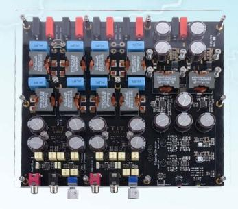
The PMP11769 reference design is a complete solution for a 700W automotive audio amplifier. The boost converter provides  $36 \text{ V} \@ 10 \text{ A}$  continuous / 20 A peak from an input voltage of 9 -16 V. It contains two Class-D amplifiers which provide  $2x \ 175 \ W \@ 4 \ Ohm \ load (left \& right channel) and <math>1x \ 350 \ W \@ 2 \ Ohm \ (subwoofer)$ .
