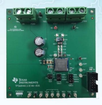
The integrated-inductor power module at the heart of this PMBus<sup>™</sup> demo is rated for 18VIN-max and 35A, and is configured for a default output of 1.2V.
