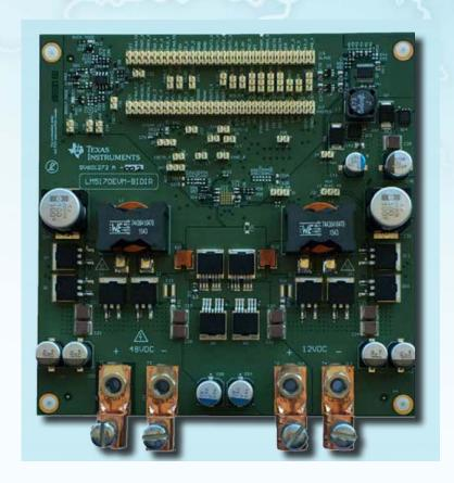
This demo utilizes a standard evaluation module to demonstrate the LM5170-Q1's ability to transfer current in either buck mode (48V to 12V) or boost mode (12V to 48V) operation by simply controlling the direction pin.
