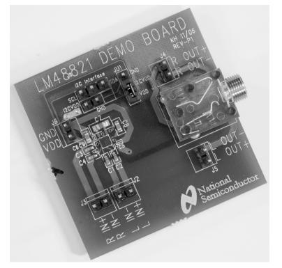
Figure 1. LM48821 Demonstration Board
