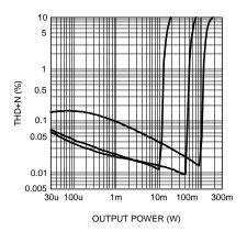
Figure 13. Stereo THD+N vs Output Power  $R_L = 32\Omega$ ,  $A_V = 0dB$ , f = 100Hzat (from left to right at 1% THD+N):  $V_{DD} = 2V$ ,  $V_{DD} = 3V$ ,  $V_{DD} = 4V$ , both channels driven and measured
