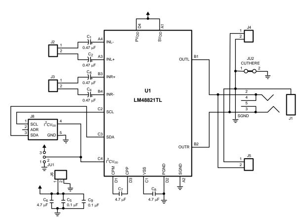
Figure 2. LM48821 Demonstration Board Schematic
