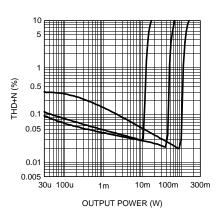
Figure 11. Stereo THD+N vs Output Power  $R_{L} = 16\Omega$ ,  $A_{V} = 0$ dB, f = 1kHz at (from left to right at 1% THD+N):  $V_{DD} = 2V$ ,  $V_{DD} = 3V$ ,  $V_{DD} = 4V$ , both channels driven and measured
