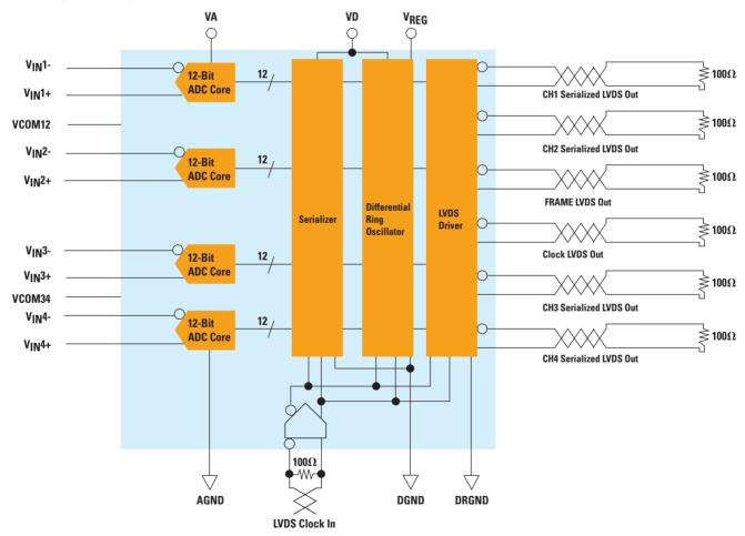
Figure 1. ADC12QS065 Simplified Block Diagram
