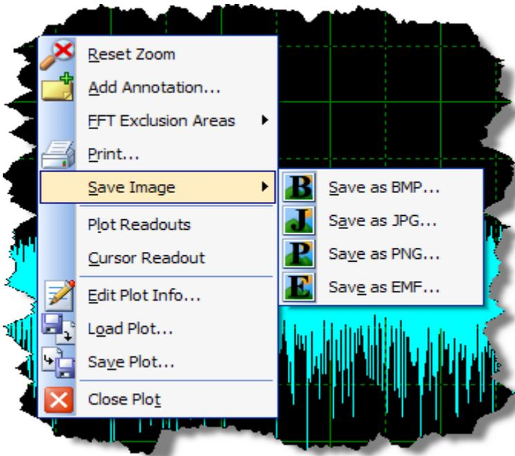
You may save images of the plot to disk in one of four different formats, as illustrated above. BMP, JPG and PNG formats are all bitmap or pixel based, meaning they won't scale well. EMP (enhanced metafile format) is a standard Windows vector based format. This means that the contents of the image are described mathematically which allows the image to scale smoothly. This is the best format to use when you need to include the image in another document.
