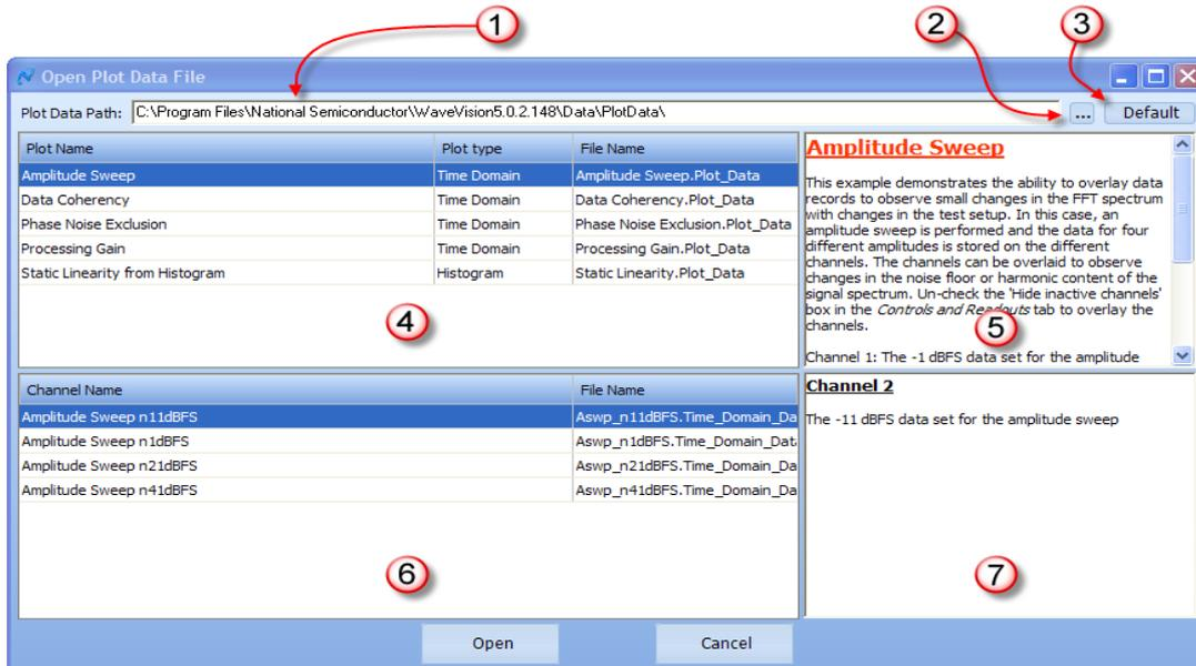
By default, the Open Plot File dialog uses the PlotData directory created when WaveVision 5 was installed. The dialog lists the plot files it finds in the PlotData directory.
