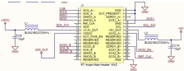
Figure 9 - LMP91050SDEVAL's J1 for SPI Signals
