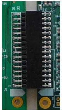
Figure 4 – LMP91050SDEVAL-to-SPIO-4 Board Connection
