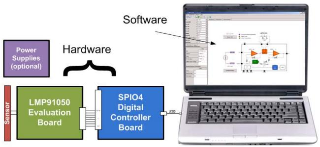
Figure 1 – Connection Diagram
