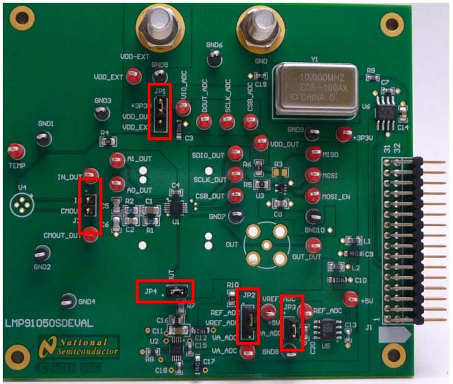
Figure 3 – Jumper Settings (Default) for voltage reading
