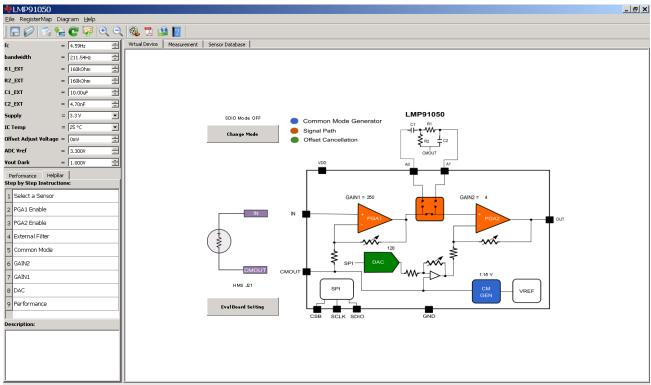
Figure 6 - Recommended LMP91050 Configuration for a voltage Reading
