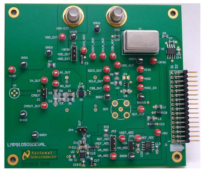
Figure 2 – LMP91050 Evaluation Board Assembly
