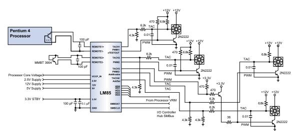
Figure 1: Typical LM85 Connection
