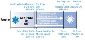
Figure 3: LM85 Fan Control Registers
