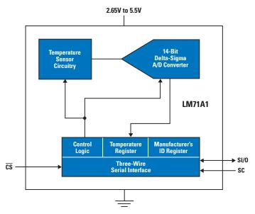
Figure 1. Simplified Block Diagram
