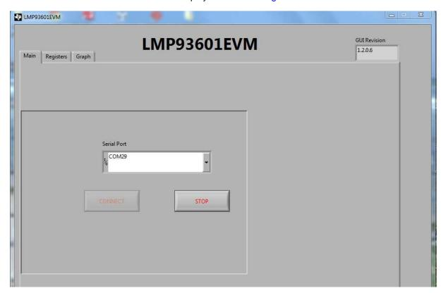
Figure 5. GUI Communication Port Selection
