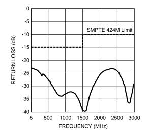
Figure 2. LMH0387 Input Return Loss
