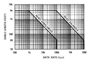
Figure 1. Data Modulation Rate vs Cable Length
