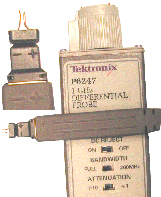
Tektronix 1GHz P6247 differential probe. Note two probe contacts and polarity indication in probe tip detail.
