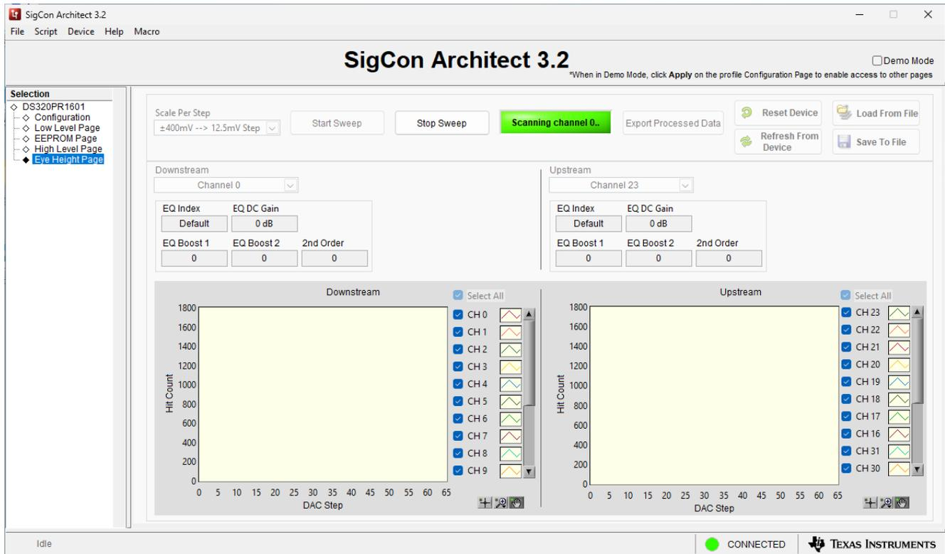
**Figure 5-2. Eye Scan Sweep Initiated, Indicated by Green Scanning Channel X Display**
