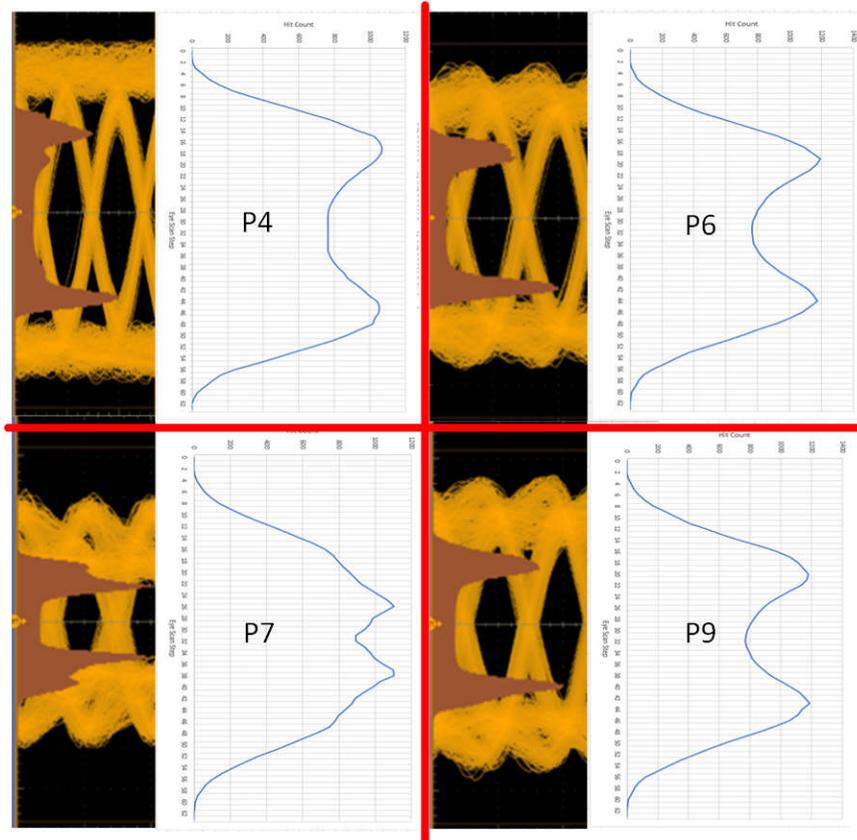
**Figure 4-2. PCIe TX Preset Comparison From Oscilloscope and Eye Scan. From Top Left to Bottom Right: TX Preset P4, P6, P7, P9**
