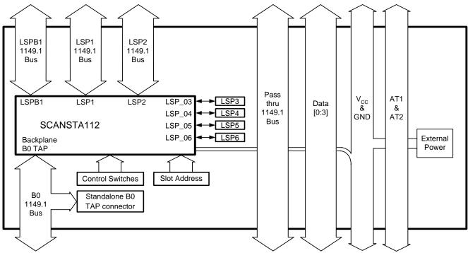
Figure 1, Basic block diagram of the STA112 Multidrop card
