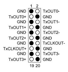
Figure 4: LVDS Output Connections (J1)
