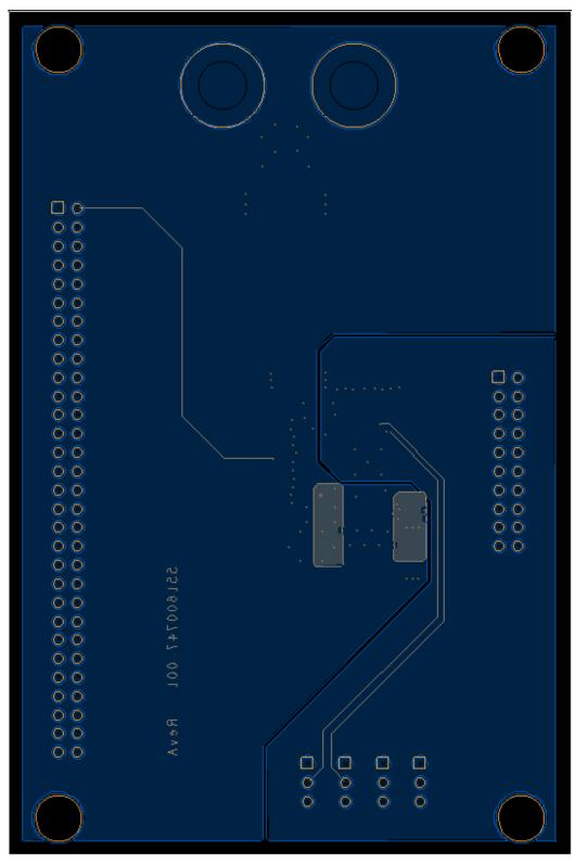
Figure 8: Bottom Layer Routing
