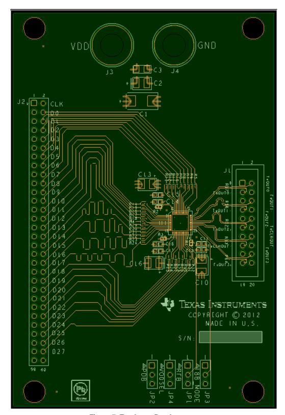
Figure 7: Top Layer Routing
