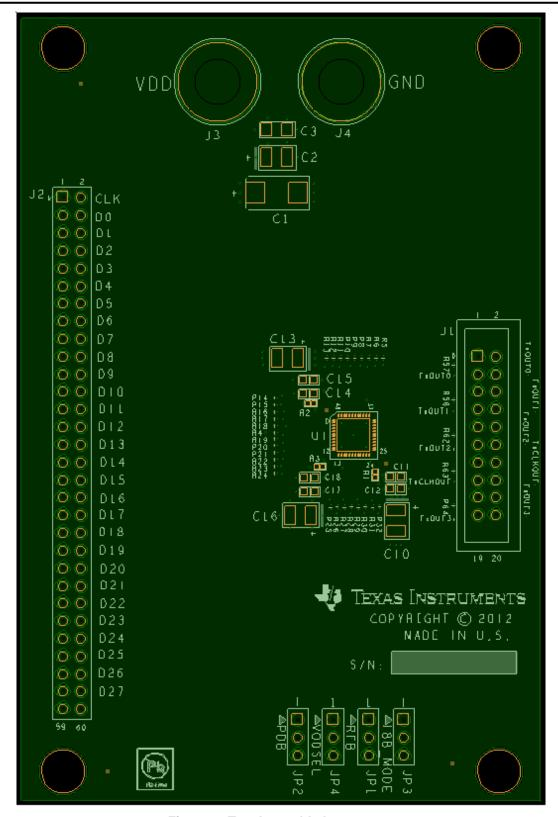
Figure 6: Top Assembly Layer
