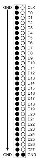
Figure 5: LVCMOS Input Connections (J2)
