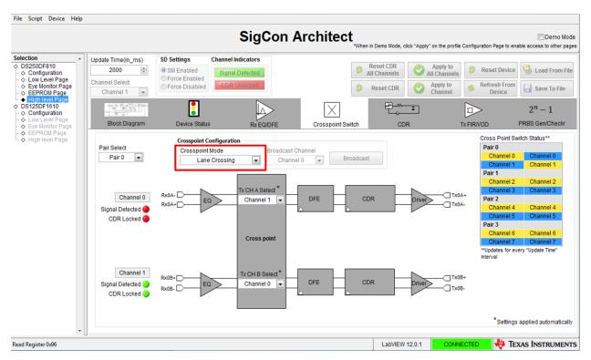
Figure 14. Cross-Point Tab, Lane Crossing Mode Selected
