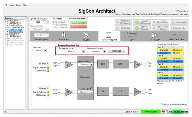
Figure 13. Cross-Point Tab, Fanout Mode Selected
