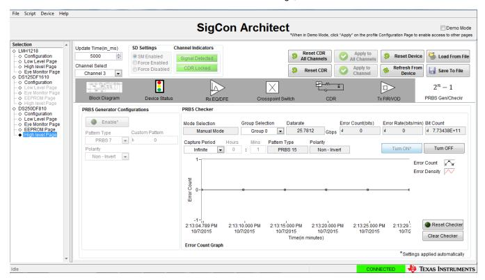
Figure 19. PRBS Tab, PRBS Checker Configuration
