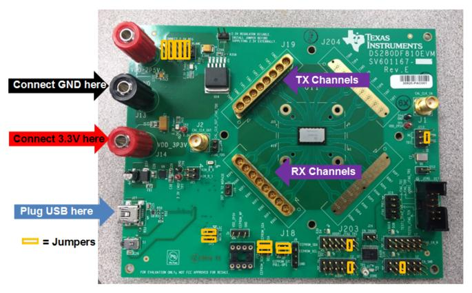
Figure 1. DS280DF810EVM, Showing Necessary Connections for Power, Signal, and USB Communications
