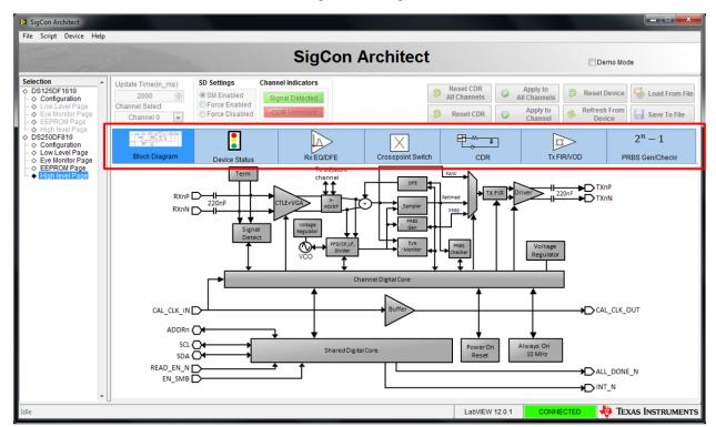
Figure 9. High-Level Page, with Block Diagram Tab Selected
