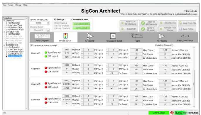
Figure 10. High-Level Page, with Device Status Tab Selected
