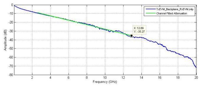
Figure 20. SDD21 Loss Characteristic of Example Test Case
