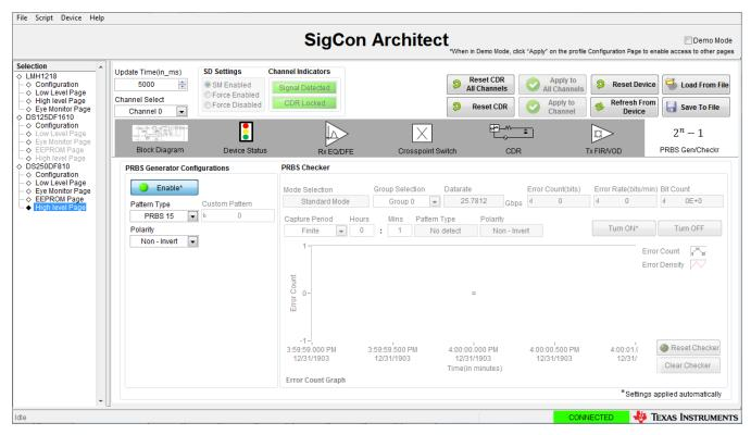
Figure 18. PRBS Tab, PRBS Generator Configuration
