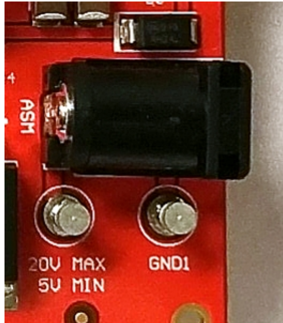
Figure 3. Onboard Power Supply Connection
