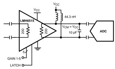
Figure 1. LMH6515 With Output Pull-Up Inductors
