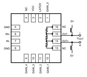
Figure 3. Using High-Gain Mode (400Ω Load)
