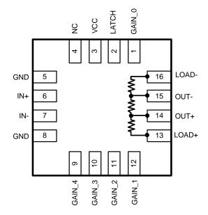
Figure 2. Internal Load Resistors
