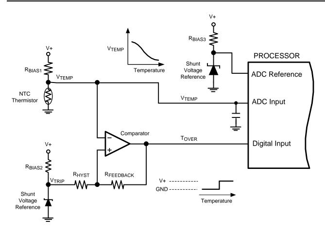
Figure 1. Classic Thermistor-based Discrete Temperature Sensor Circuit
