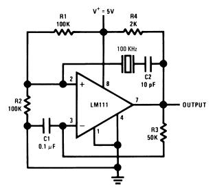
Figure 9. Crystal-Controlled Oscillator
