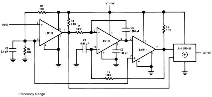
Input—5 kHz to 50 kHz Output—10 kHz to 100 kHz
