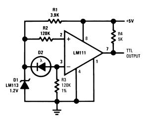
Figure 4. Precision Level Detector for Photodiode
