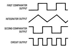
Figure 11. Waveforms for the Frequency Doubler
