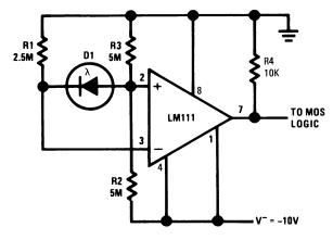
Figure 3. Level Detector for Photodiode
