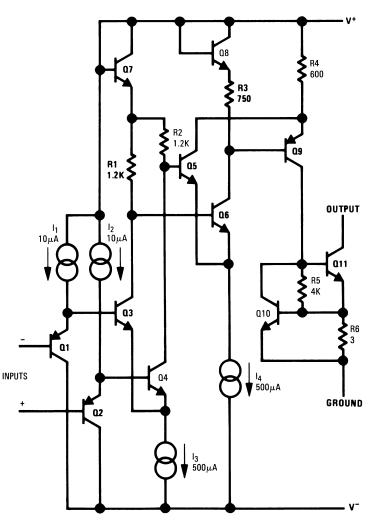
Figure 1. Simplified Schematic of the Comparator
