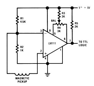
Figure 2. Zero Crossing Detector for Magnetic Transducer
