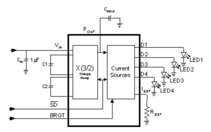
Other benefits to this type of constant current supply include higher efficiency than the double plus regulate architecture, as well as several options to actively control the brightness of the LED. Since a current mirror architecture is used, LED current for all LEDs is set by one resistor using a large amplification ratio. By using a 20:1 or greater ratio, power consumption of the system is minimized.
