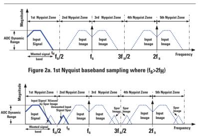
Figure 2b. 1st Nyquist sampling with no ADC input filter showing input spur  $f_s/2$  aliasing back into 1st Nyquist zone to interfere with input  $f_s/2$
