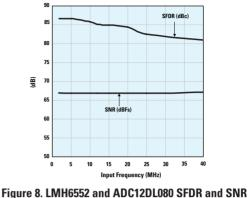
Figure 8. LMH6552 and ADC12DL080 SFDR and SNR performance vs frequency
