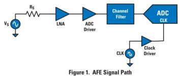
A key measure of any data-acquisition-system performance is the Effective Number Of Bits (ENOB) of resolution it delivers. The ENOB is maximized by minimizing the noise and distortion added by each stage of the AFE to the processed signal. A measure of the noise added by a particular stage is the noise factor, F, which is the total input referred noise of the stage divided by the input noise due to the previous stage. The often-quoted Noise Figure, NF, is 10 log F.
