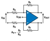
Figure 6a. Fully differential amplifier
