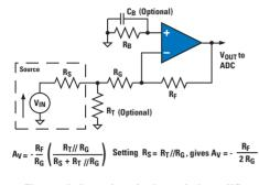
Figure 5b. Inverting single-ended amplifier
