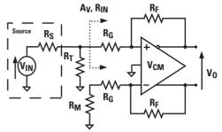
To match circuit input impedance  $R_{\rm IN}$  to source impedance  $R_{\rm S},$  set  $R_{\rm T}//R_{\rm IN}$  =  $R_{\rm S},$  with  $R_{\rm M}$  =  $R_{\rm S}//R_{\rm T}$  then
