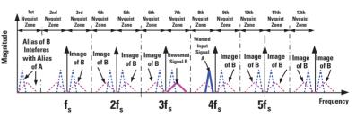
Figure 3b. Failure to bandpass filter unwanted signal B allows it to alias back to the 1st Nyquist zone and interfere with the recovery of wanted signal A
