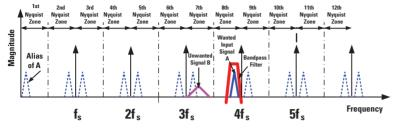
Figure 3c. Unwanted signal B prevented from aliasing B by bandpass filter around A
