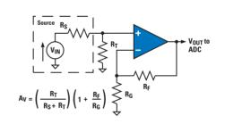
Figure 5a. Non-inverting single-ended amplifier
