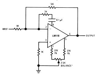
\*Balance circuit necessary for increased slew.
