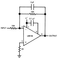
Slew and settling time to 0.1% for a 10V step change is 800 ns.
