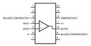
Figure 1. CDIP Package Top View See Package Number J0014A
