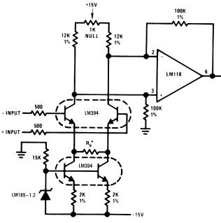
\*Gain  $\geq \frac{200 \text{K}}{\text{R}_g}$  for 1.5K  $\leq \text{R}_g \leq 200 \text{K}$
