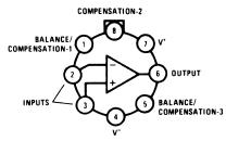
Pin connections shown on schematic diagram and typical applications are for TO-5 package.
