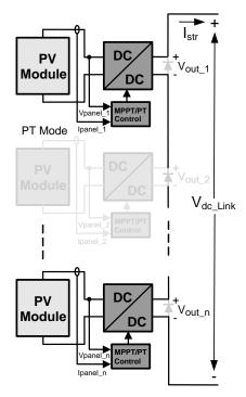
Figure 4. Panel Mode Offering Almost Lossless Energy Harvest
