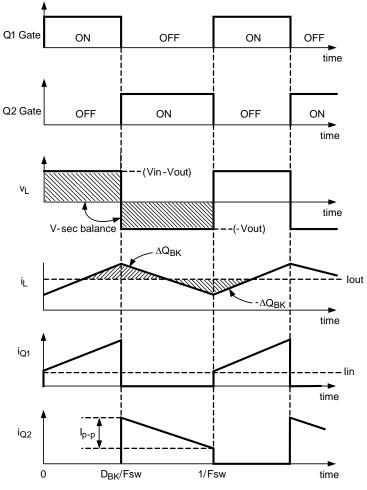
Figure 8. Buck-Only Key Waveforms
