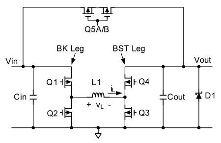
Figure 5. Buck-and-Boost Converter Topology With Panel Mode Switch
