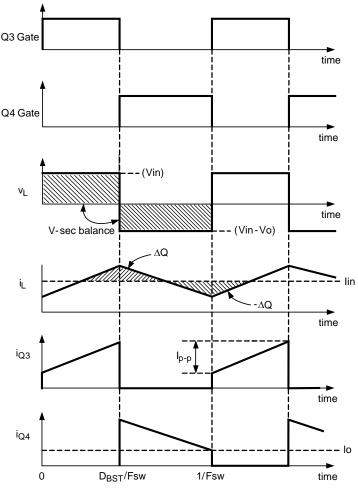
Figure 9. Boost-Only Key Waveforms
