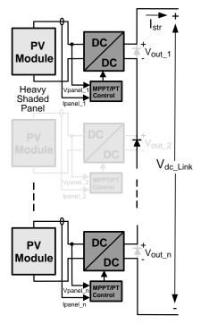
Figure 3. Output Bypass Diode Continues the String Current
