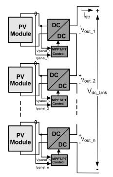
Figure 2. A String of MPPT/PM Enhanced PV Modules
