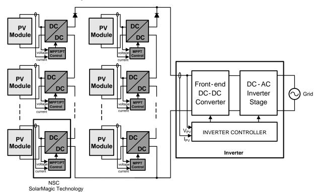
Figure 1. SolarMagic MPPT/PM Enhanced PV System Architecture
