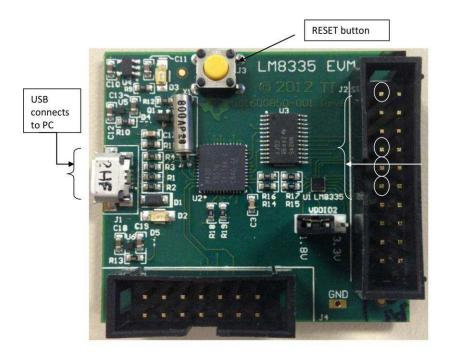
Pin 1: GND Pin 7: SCLK Pin 9: SDATA Pin 11: VIO
