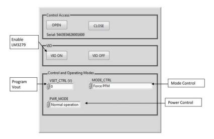
Figure 11. Programming GUI Window
