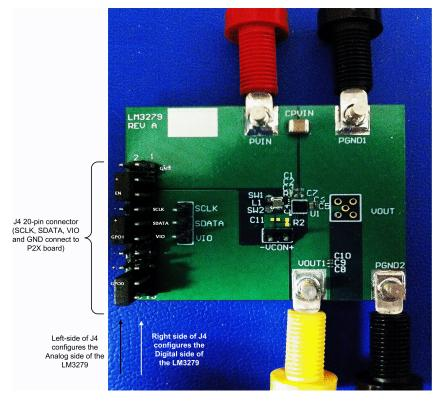
Figure 3. Photo of LM3279 Evaluation Board
