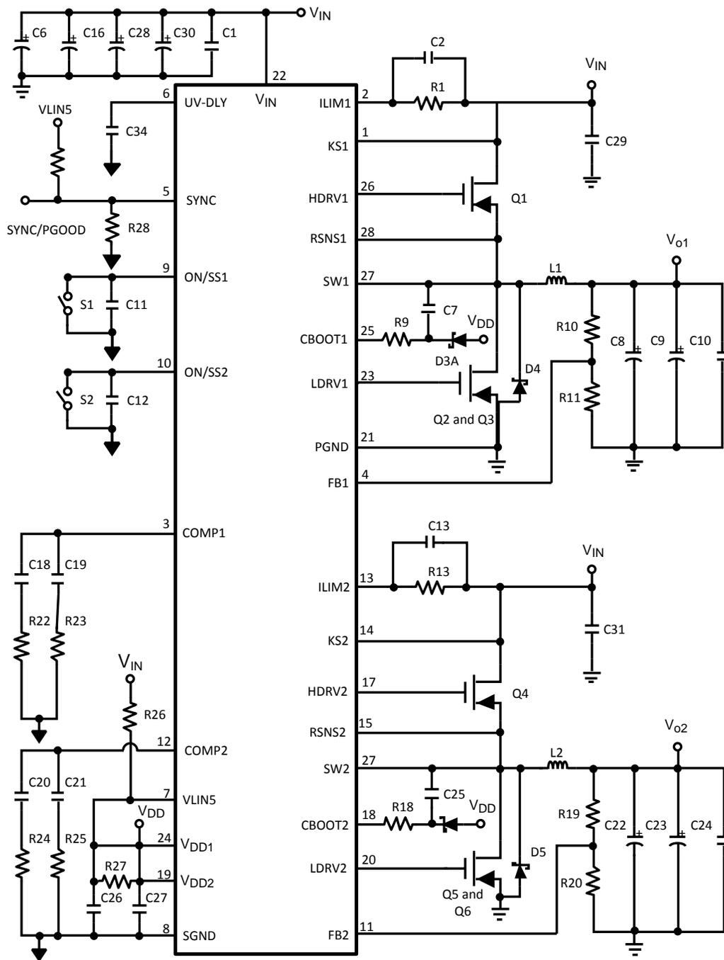
Figure 4. Complete V<sub>DS</sub> Sense Eval Board Schematic
