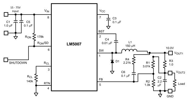
Figure 24. Low Output Ripple Configuration
