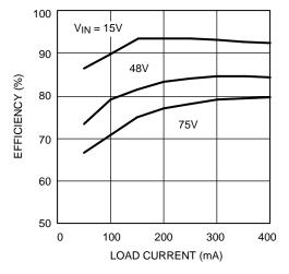
Figure 14. Efficiency vs Load Current at Vout
