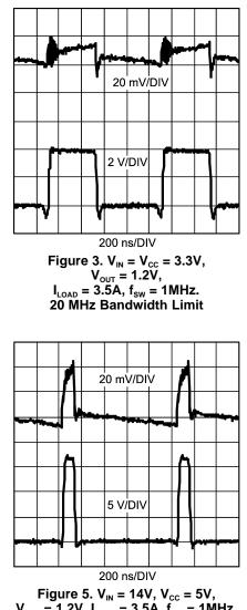
Figure 5.  $V_{IN}$  = 14V,  $V_{CC}$  = 5V,  $V_{OUT}$  = 1.2V,  $I_{LOAD}$  = 3.5A,  $f_{SW}$  = 1MHz. 20 MHz Bandwidth Limit
