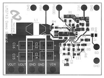
Figure 7. Top Layer and Top Overlay
