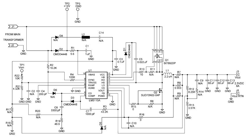
Figure 23. LM5115A AC Eval Board Schematic
