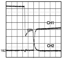
V<sub>IN</sub> = 48V; LM5115 Load = 5.0A CH1 = Lo Side Sw Gate Drive, 2V/Div. CH2 = Hi Side Sw Gate Drive, 2V/Div. Horizontal Resolution = 100 ns/Div.
