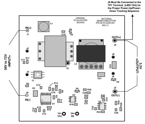
Figure 2. LM5025A Evaluation Board Top Side
