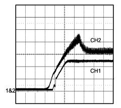
VIN = 48V; LM5115A Load = 5.0A, LM5025 Load = Open CH1 = Secondary 2.5V Output, 1V/Div.
