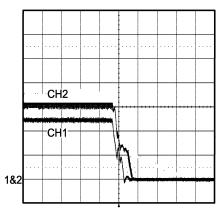
VIN = 48V; LM5115A Load = 5.0A, LM5025 Load = Open CH1 = Secondary 2.5V Output, 1V/Div. CH2 = Main 3.3V Output, 1V/Div. Horizontal Resolution = 200 µs/Div.
