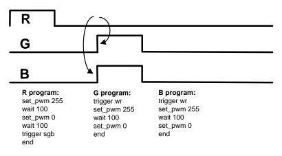
Figure 7. Sending Multiple Triggers Example
