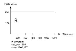
Figure 3. Using Ramp Command as Wait
