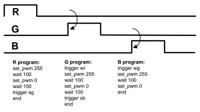
Figure 6. Basic Triggering Example
