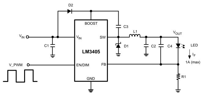
Figure 2. PWM Dimming of LEDs by Applying a PWM Signal to the EN/DIM Pin
