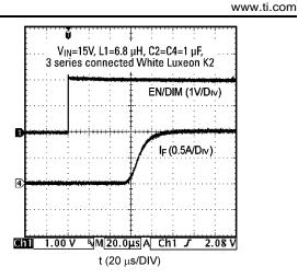
Figure 4. Startup Response of the LM3405 to an EN/DIM Signal with I<sub>F</sub> Set at 1A
