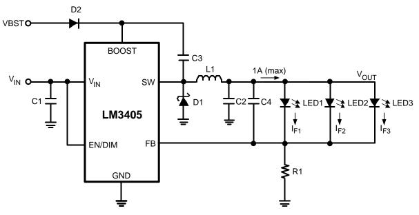
Figure 7. Driving Multiple LEDs in Parallel
