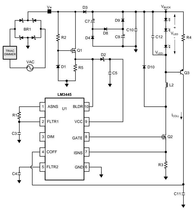
Figure 1. Simplified LM3445 Schematic
