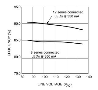
Figure 2. Efficiency Plot
