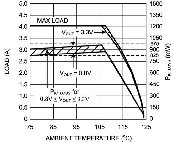
Figure 6. Current Derating vs. Ambient Temperature LMZ10504EXT,  $V_{IN} = 5.0V$ ,  $\theta_{JA} = 20^{\circ}C/W$
