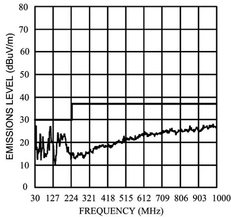
**Figure 22. Radiated Emissions (EN55022, Class B)**
