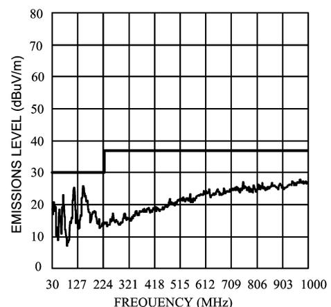
Figure 21. Radiated Emissions (EN55022, Class B)
