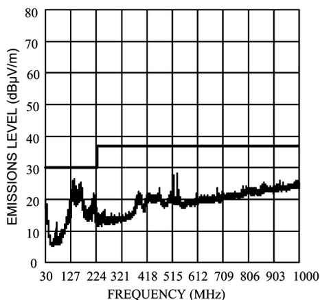
Figure 20. Radiated Emissions (EN55022, Class B)
