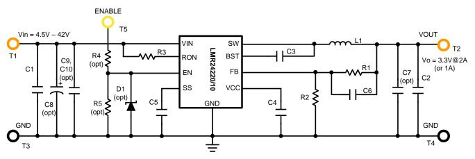
Figure 3. LMR24210/20 Evaluation Board Schematic
