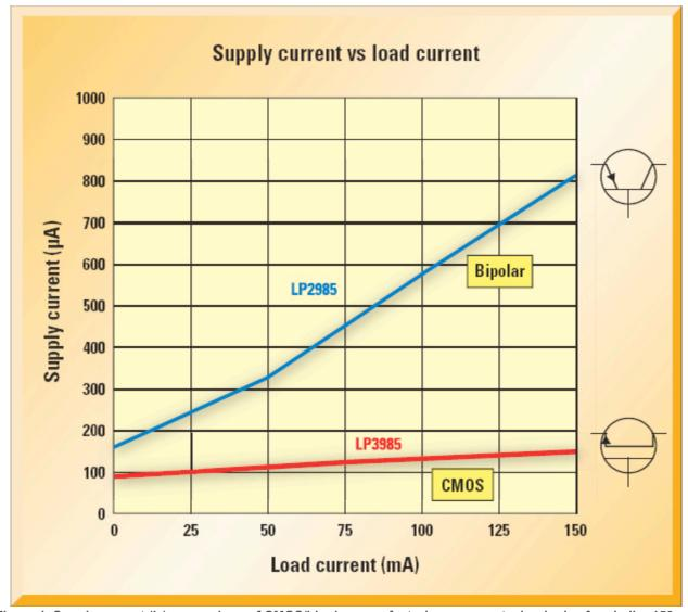
Figure 1. Supply current (I<sub>q</sub>) comparison of CMOS/bipolar manufacturing process technologies for similar 150 mA LDOs over full load-current range
