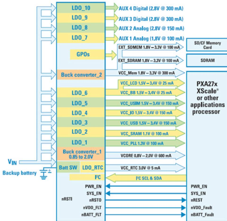
Figure 1. LP3970 Application diagram
