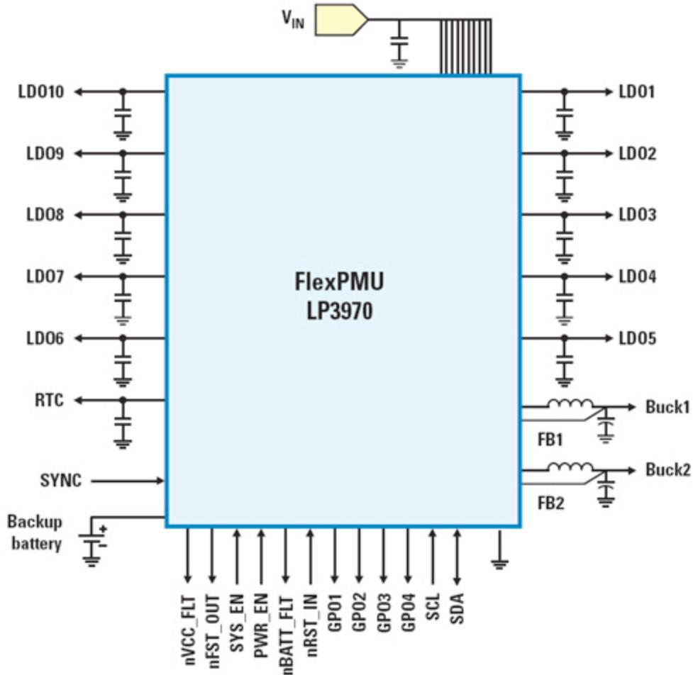
Figure 2. LP3970 functional schematic
