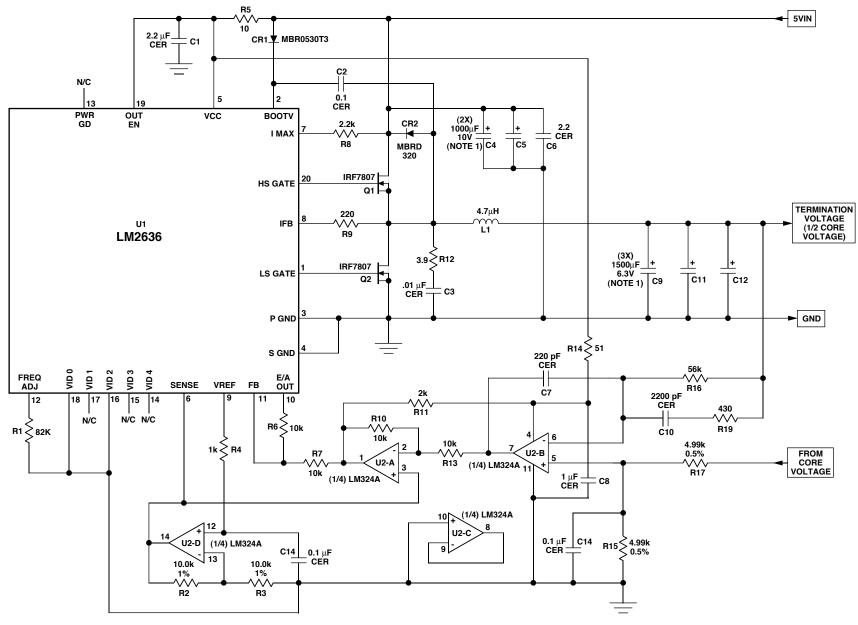
NOTE 1. USE LOW ESR ALUMINUM ELECTROLYTIC CAPACITOR SUITABLE FOR 300K HZ SWITCHING APPLICATIONS.
