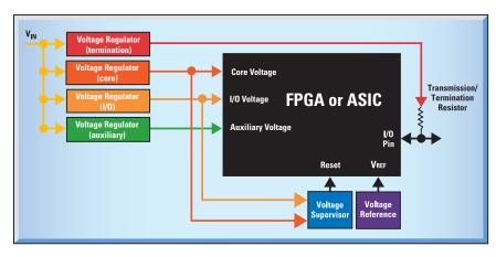
Figure 1: Typical FPGA or ASIC power management requirements
