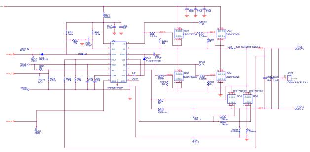
Figure 12. TPS92641 Green LED Driver Schematic
