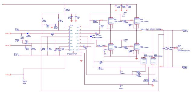
Figure 13. TPS92641 Blue LED Driver Schematic
