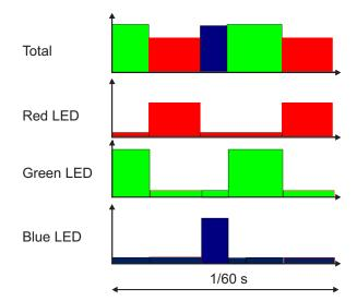
Figure 3. Brightness Turbo Slightly Turned on all LEDs at all Times
