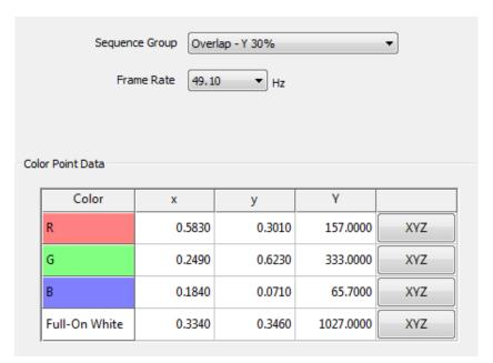
Figure 10. Smaller Color Gamut When Brightness Turbo Enabled
