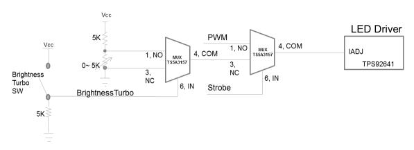
Figure 4. IADJ Control of Brightness Turbo
