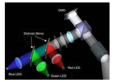
Figure 1. Optical Layout of DLP® LED Projector
