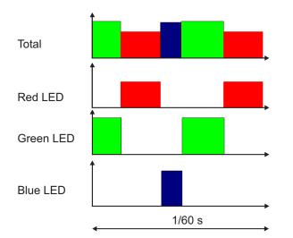
Figure 2. Conventional LED Driving Scheme in 60 Hz Video
