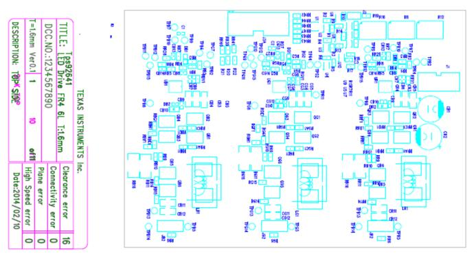
Figure 17. PCB Top View With Component
