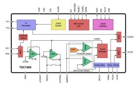
Figure 2. TDC1000-Q1 Block Diagram
