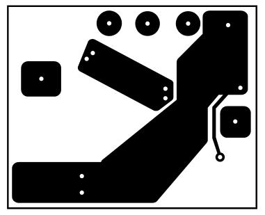
Figure 19. Solder Side PC Board Layout
