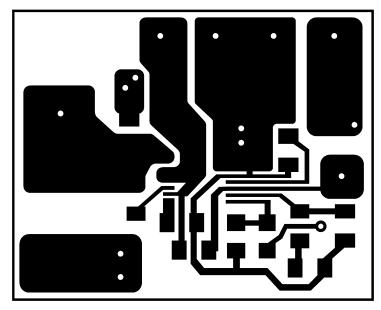
Figure 18. Component Side PC Board Layout
