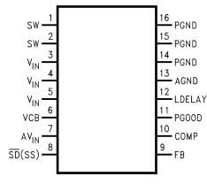
Figure 14. 16-Lead TSSOP (PW) See Package Number PW0016A
