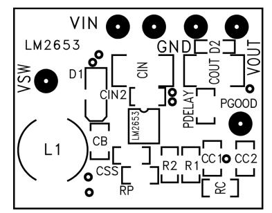
Figure 17. Component Placement Guide
