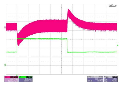
The photo below shows the 13.2V output voltage (ac coupled) when the load current is stepped between 2A and 3A. Vin = 12V. (100mV/DIV, 1A/DIV, 1mS/DIV)
