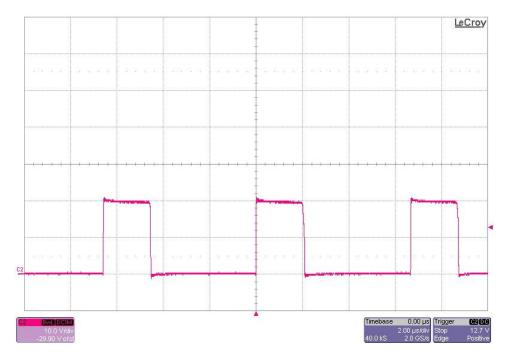
The photo below shows the FET switching voltage (TP4) for an input voltage of 16V and a 1.15A load. The converter is operating in DCM. (10V/DIV, 2uS/DIV)
