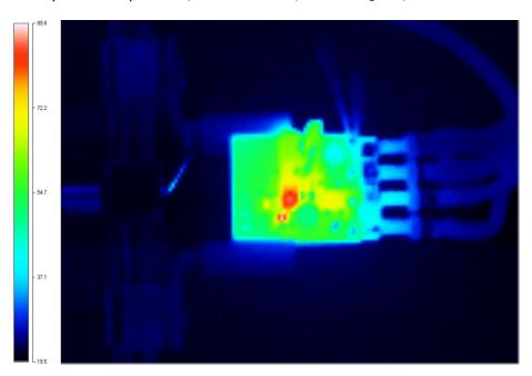
The Mosfet and Shunt resistor are the hottest items. Heat-sinking recommended.
