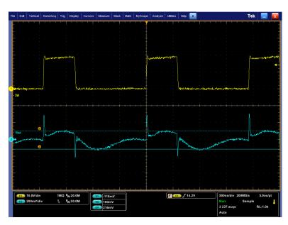
12Vin, 12Vout @ 4A load current. (~160mV p-p Ripple)
