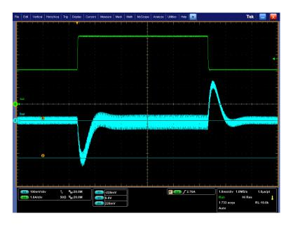
16Vin @ 2A to 4A, 100mA/ $\mu$ s, Pulse f @ 100 Hz, 50% duty cycle, 12V out. Load Step on/off.
