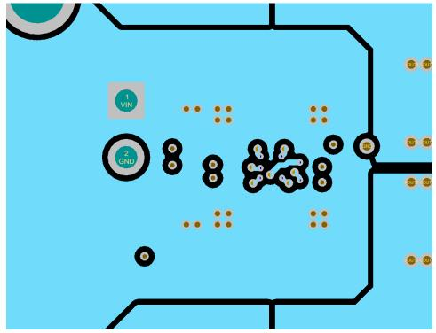
Plane kept intact around the LP8758 device.
