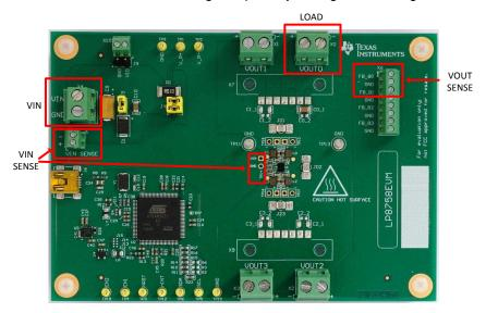
Figure 4. Connections for Efficiency Measurement
