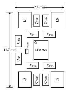
Figure 6. Component Placement near the LP8758 Device
