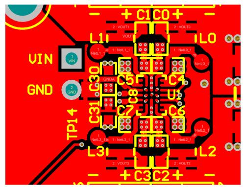
Input capacitors are placed close to the LP8758 and routed on top layer. GND nets are connected to the GND plane (2nd layer) with microvias. VIN nets are connected to the VIN plane (3rd layer) with vias in pads of the input capacitors. VOUT pads of the output capacitors and inductors are connected together with large copper area.
