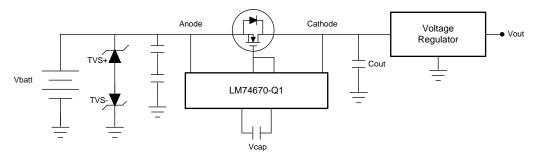
Figure 1. LM74670-Q1 Typical Application Circuit
