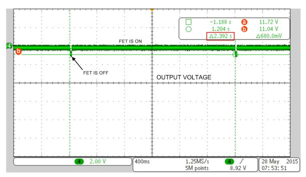
Figure 6. The LM74670-Q1-SQEVM Output voltage waveform
