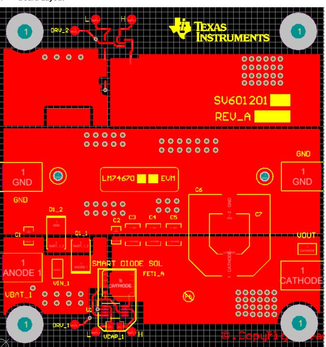
Figure 7. Top Assembly Layer
