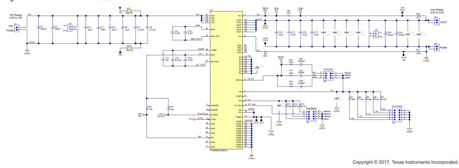
Figure 6-1. TPSM846C24EVM Schematic
