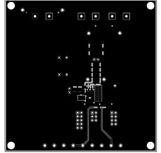
Figure 8-4. Layer 3 Copper (Top View)
