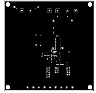
Figure 8-3. Layer 2 Copper (Top View)
