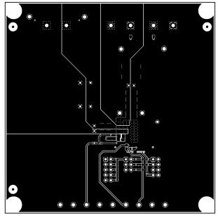
Figure 8-7. Bottom-Side Copper (Top View)
