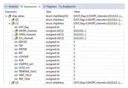
Figure 4-2. Example of Watching Expression chip\_status Without Errors for TPS929120-Q1
