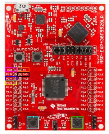
Figure 3-1. Connections on MSP-EXP430F5529LP
