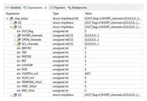
Figure 4-4. Example of Watching Expression chip\_status With Low Supply for TPS929120-Q1
