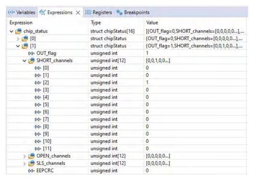
Figure 4-3. Example of Watching Expression chip\_status with Short Fault for TPS929120-Q1
