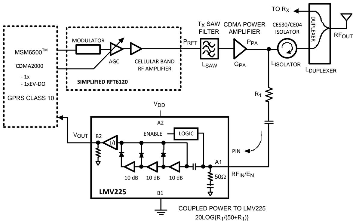
Figure 5. Single-Band CDMA2000 T<sub>x</sub> Architecture
